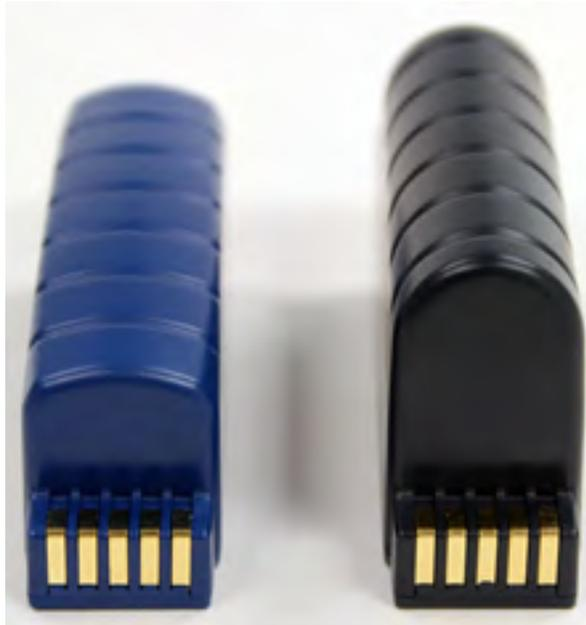
Figure 2: Talkman A700 Standard and High Capacity Batteries
